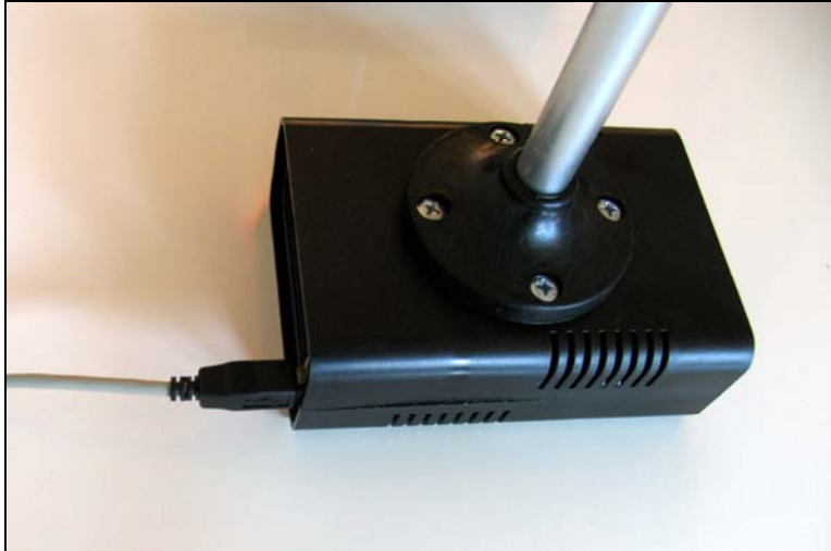
Figure 1 USB cable connected to the back of the Infolight
